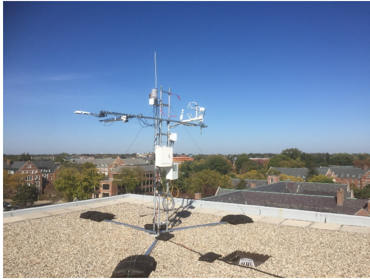
Example of a rooftop EC installation at the Michigan State University campus (PI: Jiquan Chen).
